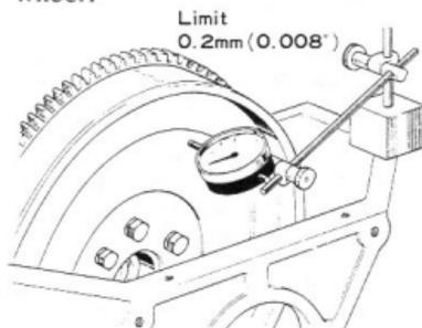
Fig.3-40 Measuring Flywheel Run-Out X4963
