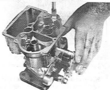
Fig.5-43 Removing Primary V0574 Main Air Bleeder
