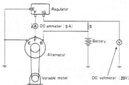
Fig. 8-43 Test Circuit X0362
