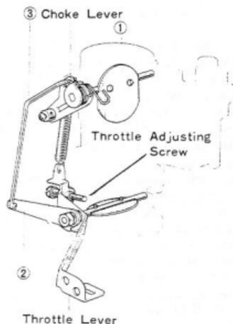
Fig. 5-7 Choke & Fast Idle System
