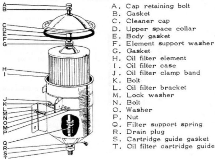
Fig.6-9 Oil Filter Components
