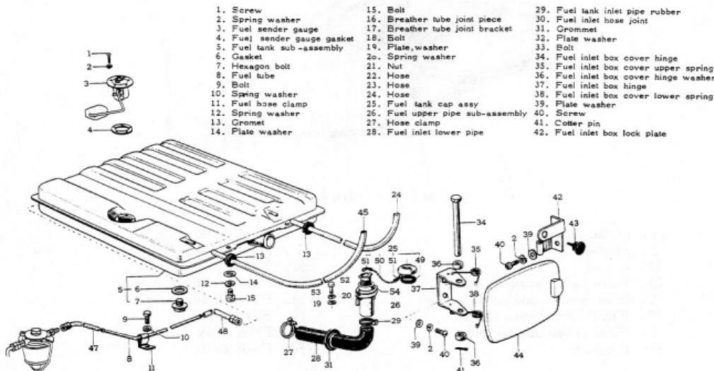
Fig. 5-103 Fuel Tank Components for FJ55V
