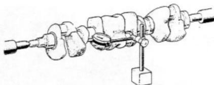
Fig.3-30 Measuring Crankshaft Bend X4952
