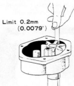
Fig.6-4 Checking Drive X5041
