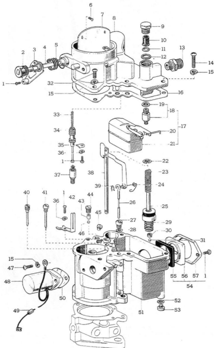
Fig.5-11 Carburetor Components
