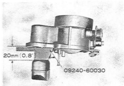
Fig. 5-24 Lowered Position V4367
