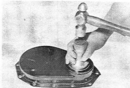
Fig.3-42 Installing Crankshaft Front Oil Seal V0550
