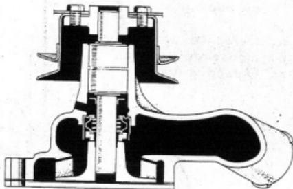
Fig.7-3 Water Pump Cross G1315 Section
