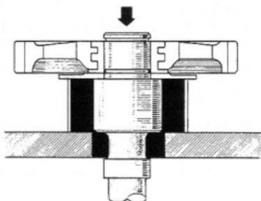
Fig. 3-35 Camshaft Timing Gear Removal X4960
