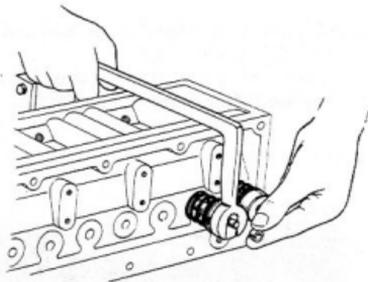
Fig.3-7 Removing Valve X4929 Spring Retainer Locks
