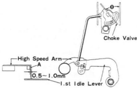
Fig.5.97 Reloader Adjustment 11345
