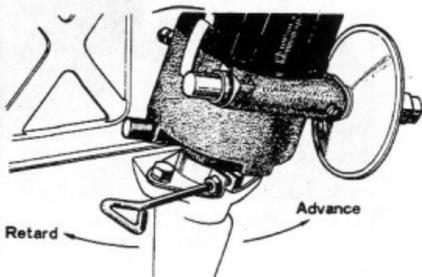
Fig. 2-7 Ignition Timing Adjustment X4920
