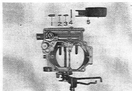
Fig. 5-76 Removing Flat 01915
