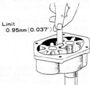
Fig.6-5 Checking Backlash X5042
