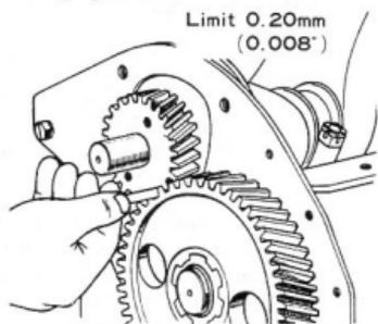
Fig.3-52 Measuring Timing X4958 Gear Backlash
