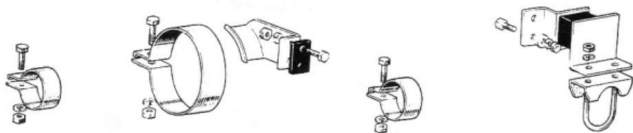
Fig.4-7 Exhaust System Components (FJ-LHD)
