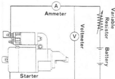
Fig.8-24 Testing Circuit G0154
