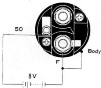
Fig.8-13 Holding Coil Test G0722
