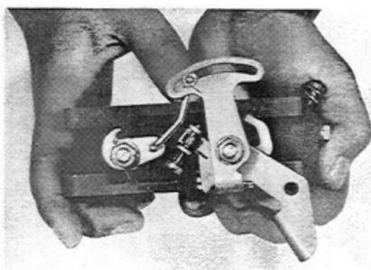
Fig.5-49 Throttle Valve V0799
