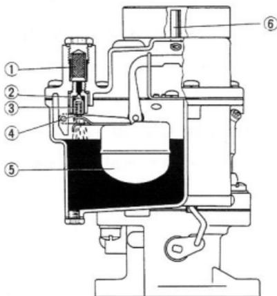
Fig.5-2 Float Chamber & G1316 Air Vent System
