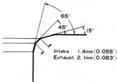
Fig. 3-13 Valve Seat Angle X4934
