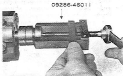
Fig.8-31 Removing Rear Bearing V1139
