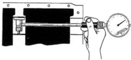
Fig. 3-36 Measuring Camshaft Bearing Bore X4948
