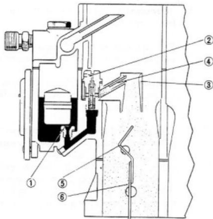
Fig.5-33 Secondary High Speed System X4994
