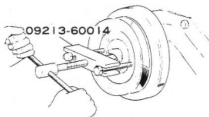
Fig.3-3 Removing Crankshaft Pulley X4925
