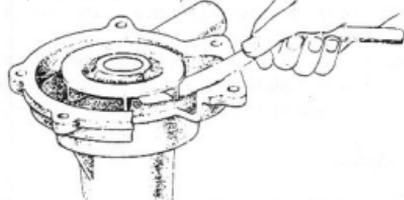
Fig. 7-7 Checking Clearance X4917
