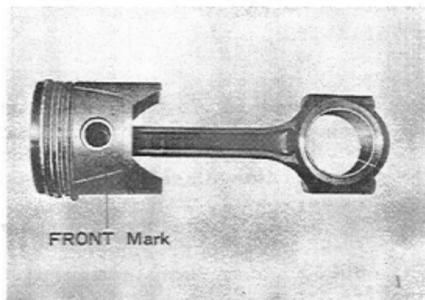
Fig. 3-44 Connecting Rod & V4352 Piston
