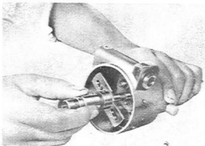
Fig. 8-49 Removing Distributor Cam W0866
