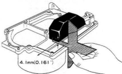
Fig. 5-78 Flat Raised 11334 Position Measurement
