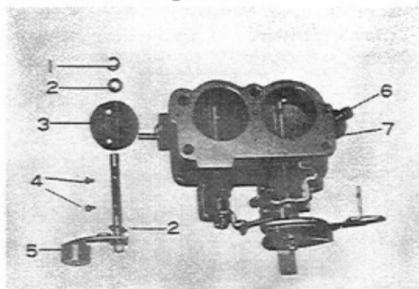
Fig. 5-73 Disassembling 01912 High Speed Valve
