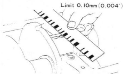
Fig.3-32 Measuring Oil Clearance X4956
