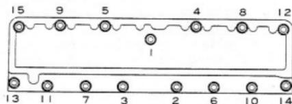
Fig.3-56 Tightening Sequence X4969
