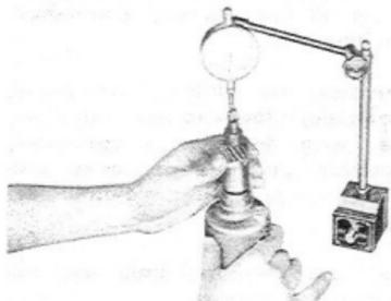
Fig.8-52 Checking Thrust Clearance V3681
