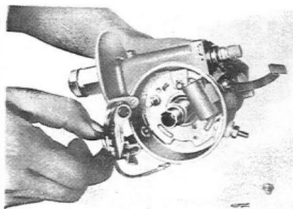
Fig. 8-47 Removing Breaker W0863 Arm & Point Plate
