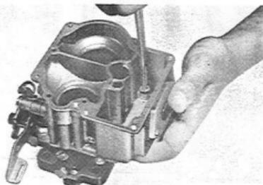
Fig.5-46 Removing Secon- V0796 dary Main Jet
