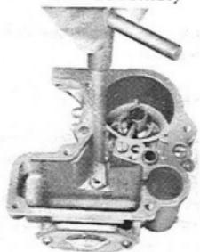
Fig. 5-17 Removing Main Jet V4364
