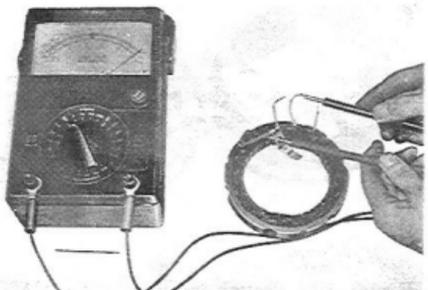
Fig. 8-35 Testing Stator Coil for Open Circuit V1145
