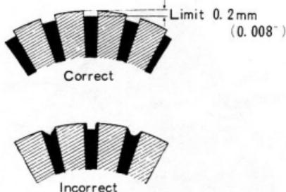
Fig. 8-6 Commutator Mica Depth X3719
