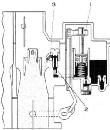
Fig. 5-35 Accelerating System X4996
