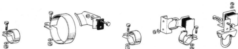
Fig.4-6 Exhaust System Components (FJ-RHD)
