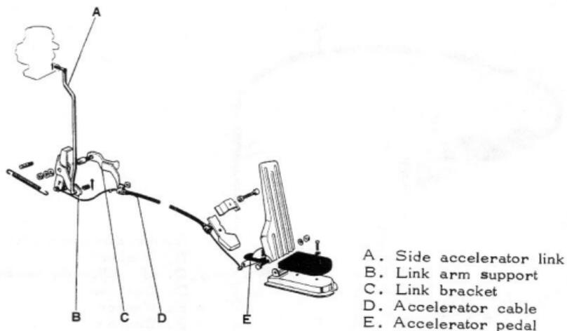
Fig. 5-113 Accelerator Linkage OLD (FA LHD) X5037
