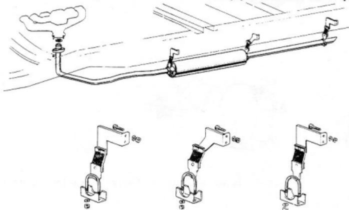
Fig.4-5 Exhaust System Components (FA series)
