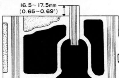
Fig. 3-11 Valve Stem Guide X4932 Extrusion (Intake)
