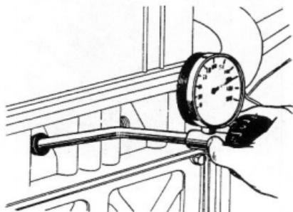
Fig. 2-10 Testing Compression Pressure X4923
