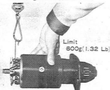
Fig.8-16 Checking Brush V4374
