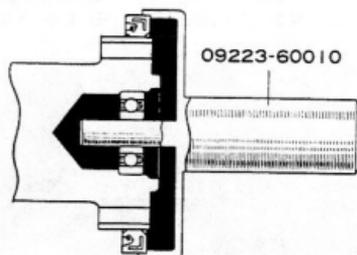
Fig.3-43 Oil Seal G1570 Installation
