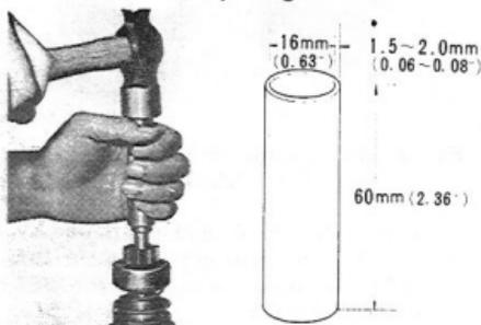
Fig. 8-5 Removing Starter Clutch V1134 X3718
