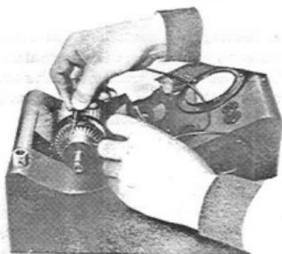
Fig. 8-9 Testing Coil for Open Circuit V2188
