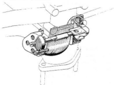
Fig.4-4 Heat Control Valve Y5720
