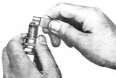
Fig.8-59 Adjusting Spark Plug Gap V2165
