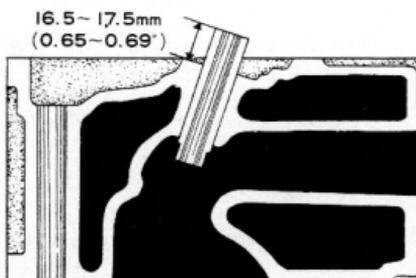
Fig. 3-12 Valve Stem Guide X4933 Extrusion (Exhaust)
