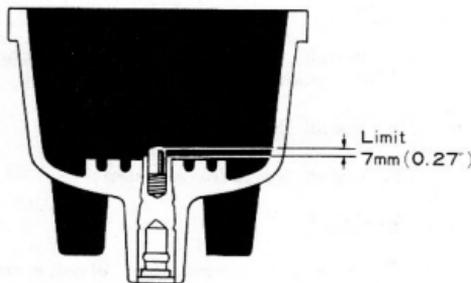
Fig.8-51 Carbon Protrusion X2936
