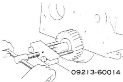
Fig.3-5 Removing Crankshaft Timing Gear X4927
