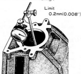
Fig.3-41 Checking Surface X4964 Parallelism
