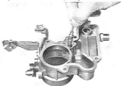
Fig. 5-13 Removing Power V4360
