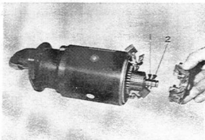
Fig.8-20 Installing Brush Holder V4376
