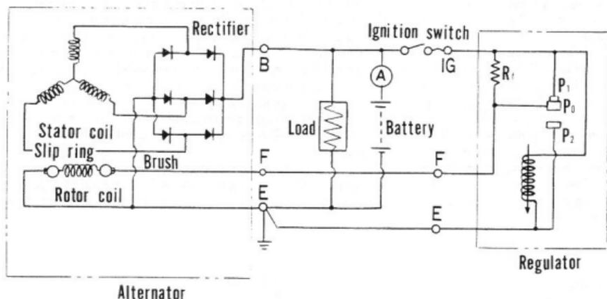
Fig.8-26 Alternator Generating Circuit
