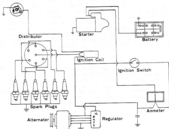
Fig.8-1 Wiring Diagram of Engine Electrical System
