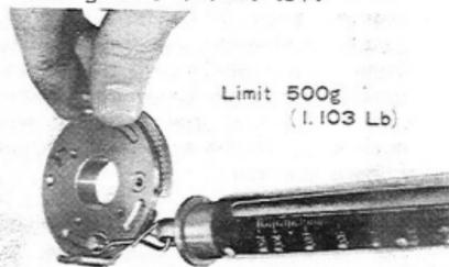
Fig.8-53 Checking Operating Resistance V1168
