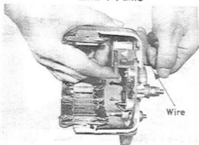
Fig. 8-41 Installing Wire V0218
