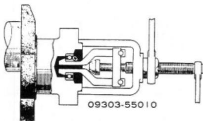
Fig.3-39 Clutch Pilot Bearing Removal G1569
