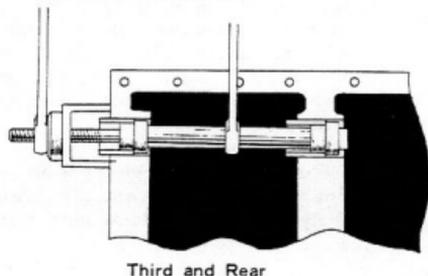
Fig.3-38 Camshaft Bearing X4950 Removal
