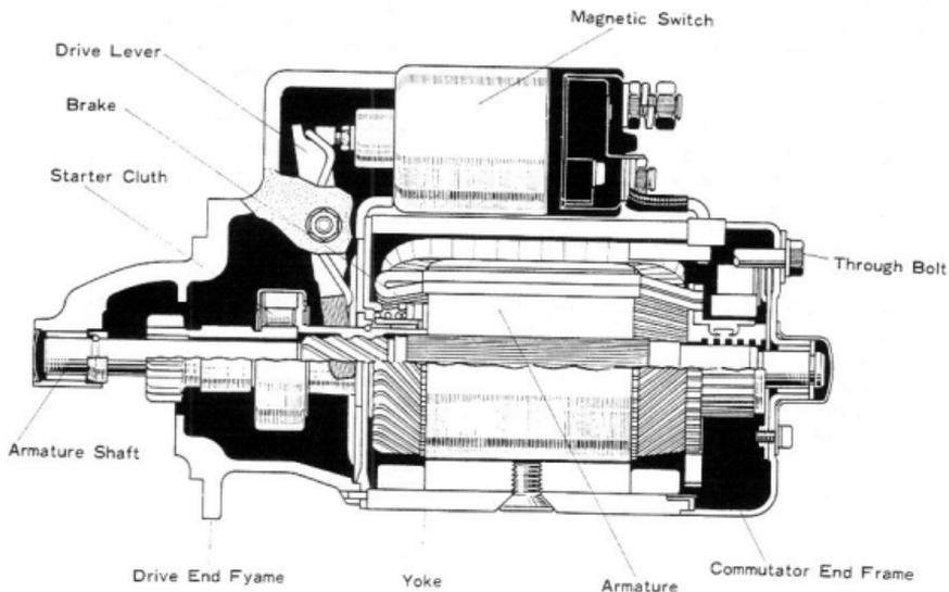
Fig.8-2 Cross Sectional View of Starter
