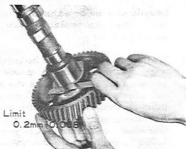
Fig.3-34 Measuring Thrust V3171 Clearance
