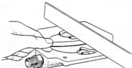
Fig.6-6 Checking Gear X5043
