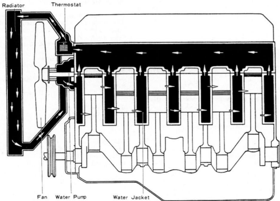
Fig.7-1 Cross Section of Cooling System
