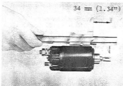
Fig.8-14 Checking Moving Stud W8636
