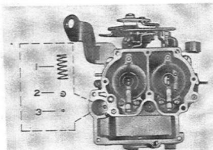
Fig. 5-65 Removing Pump Spring 01904
