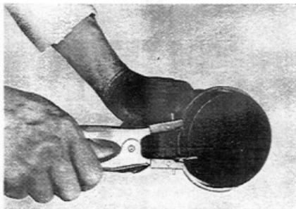
Fig.3-6 Removing Piston W0461 Rings
