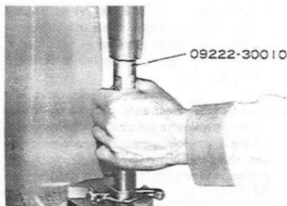
Fig.3-18 Replacing Rocker V3135
