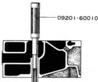
Fig.3-10 Valve Stem Guide Removal X4931
