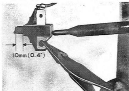
Fig.8-36 Replacing Brush V0216
