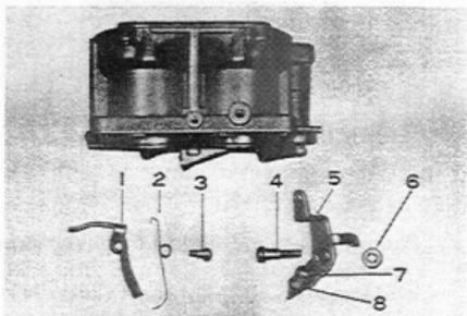
Fig. 5-85 Installing Levers 01911
