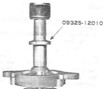
Fig. 8-40 Installing Drive End Frame V1150
