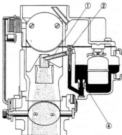
Fig. 5-4 High Speed System G1317
