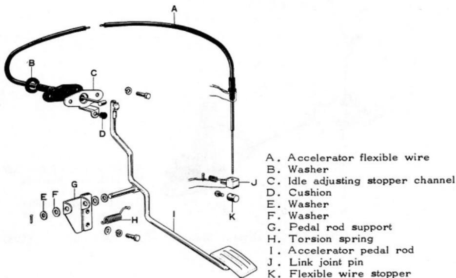
Fig. 5-111 Accelerator Linkage (FJ55V LHD)
