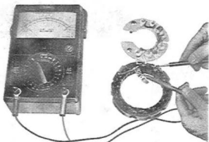
Fig. 8-34 Testing Stator Coil Insulation V1142
