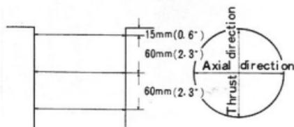
Fig.3-21 Measuring Points X0313 of Cylinder Bore
