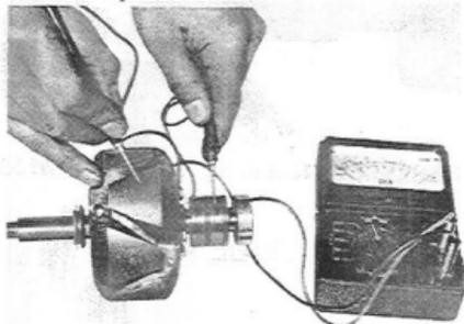
Fig. 8-33 Testing Rotor Coil for Ground V2197
