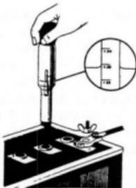
Fig.2-1 Checking Battery X4916
