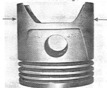
Fig.3-22 Measuring Piston V4350 Diameter
