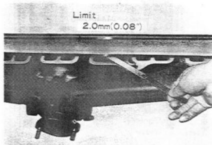
Fig.4-3 Checking Manifold Distortion V4356
