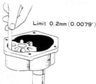
Fig.6-3 Checking Driven X5040 Gear Clearance
