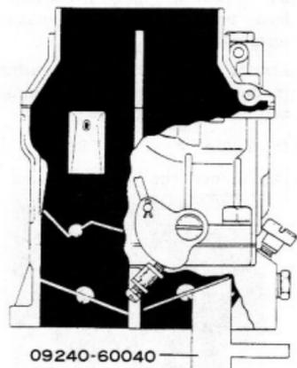
Fig.5-57 Fast Idle X5027-A Adjustment
