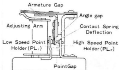
Fig.8-45 Checking Point Cap
