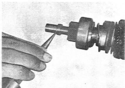
Fig.8-17 Punching Stop V1136
