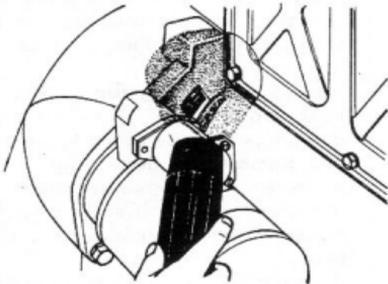
Fig. 2-6 Ignition Timing Inspection X4919
