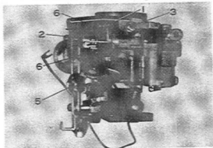
Fig. 5-63 Removing Pump Arm with Link 01902
