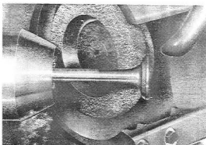
Fig.3-15 Grinding Valve V0716
