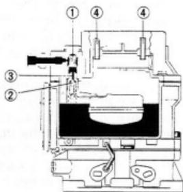
Fig. 5-30 Float Chamber & X4991
