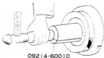
Fig.3-55 Installing Crankshaft Pulley X4955
