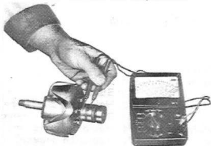
Fig. 8-32 Testing Rotor Coil V1296
