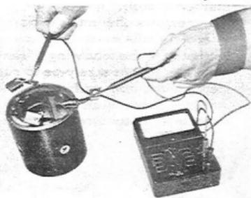
Fig. 8-10 Testing Field Coil V4371 for Open Circuit
