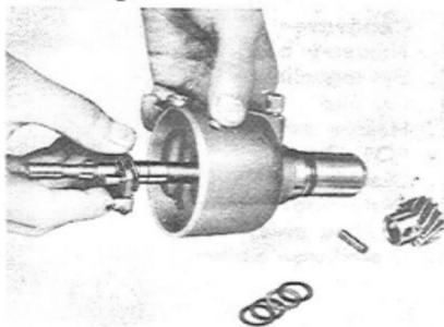
Fig. 8-50 Removing Shaft V3680
