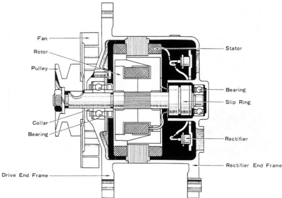
Fig.8-25 Cross Sectional View of Alternator
