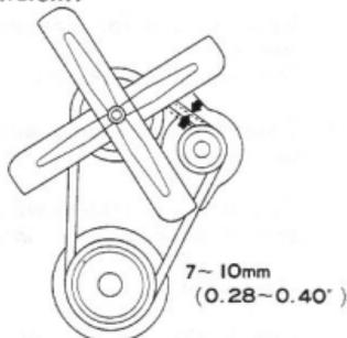
Fig. 2-2 Checking "V" Belt Tension G1567
