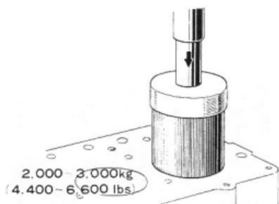
Fig.3-24 Installing Cylinder X1700 Sleeve
