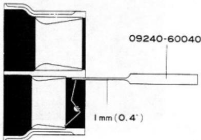
Fig.5-56 High Speed X5000-A Valve Adjustment
