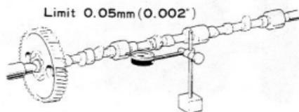
Fig.3-33 Checking Camshaft for Bend X4947
