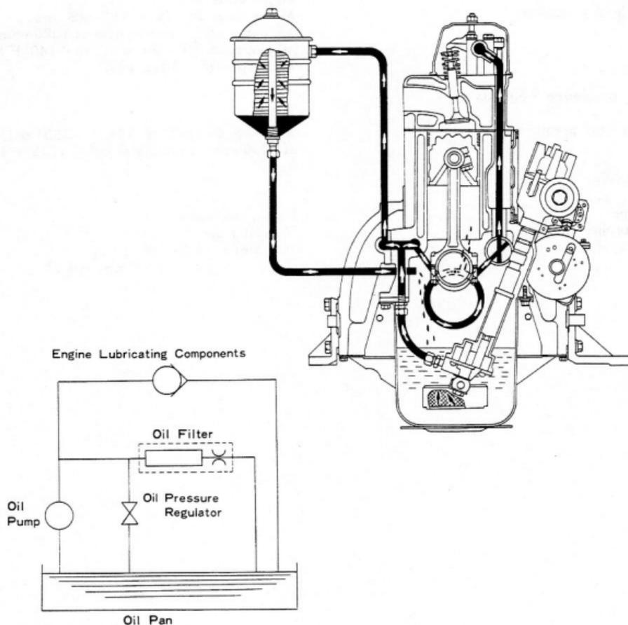
Fig.6-1 Lubricating System
