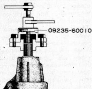
Fig.7-4 Pulley Seat Removal X5049
