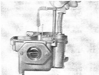
Fig. 5-14 Removing Lifter V4361
