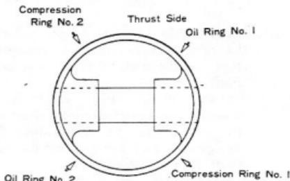
Fig. 3-49 Spacing Piston X4957 Ring Gaps
