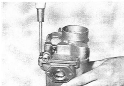
Fig. 5-12 Removing Air-horn V4359
