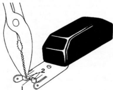
Fig. 5-80 Flat Tab 11336 Adjustments
