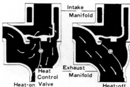
Fig.4-2 Heat Control Valve X4976 Operation
