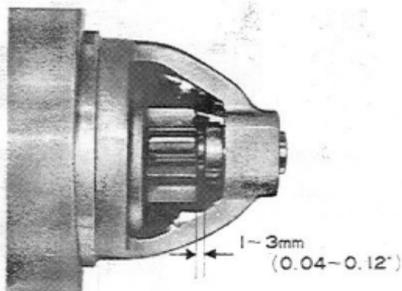
Fig.8-23 Starter Clutch Pinion Clearance W8647
