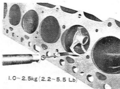
Fig. 3-23 Measuring Piston V4351 to Cylinder Clearance
