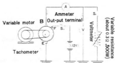
Fig. 8-42 Output Test Circuit Y5120
