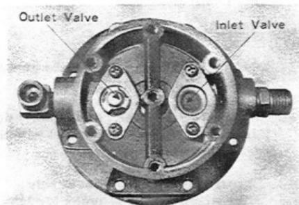
Fig. 5-100 Valve Installation V4368
