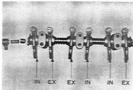
Fig. 3-48 Valve Rocker Mechanism V4354
