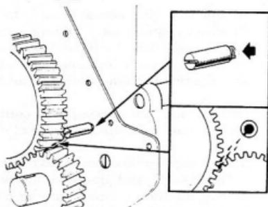
Fig.3-54 Timing Gear Oil X4968 Nozzle
