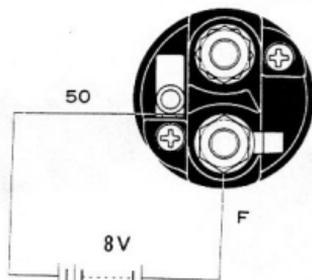
Fig.8-12 Pull-in Coil Test G0721
