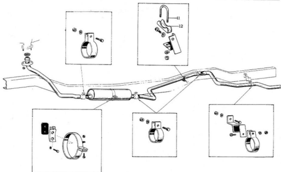
Fig.4-8 Exhaust System Components (FJ-55V)
