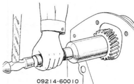
Fig.3-50 Installing Crankshaft Timing Gear X4954
